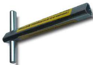
Emergency key to open/close the platform shaft door (“delta” triangle)
